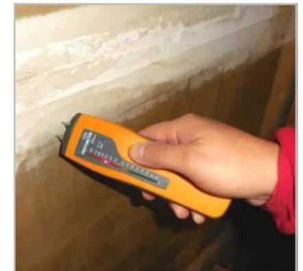
Technician checking moisture in sheetrock wall.
